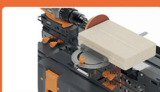
13 place wood piece onto the surface, whilst you guide the wood with the protractor for precise measurements
