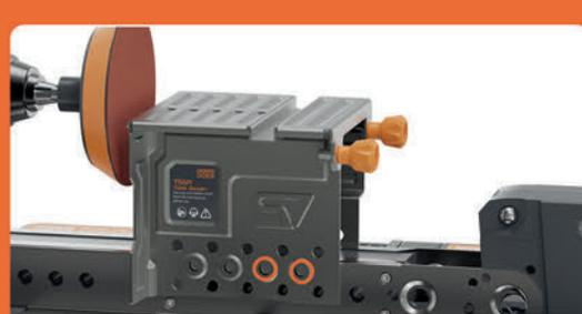
8 Align the holes same as seen on the diagram (orange circles) and secure the 3 screws
