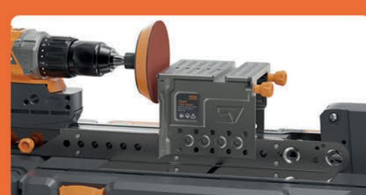
7 Align the sanding table near the mounted sanding pad
