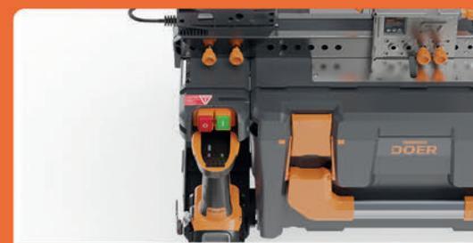
11 Insert ONE(1)Grip with Battery pack attached or AC/DC Converter on to the Charging Dock
