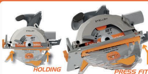
6 press the rear end of the Table Saw Shield support until hear it is securely held in place while holding the front end firmly.
