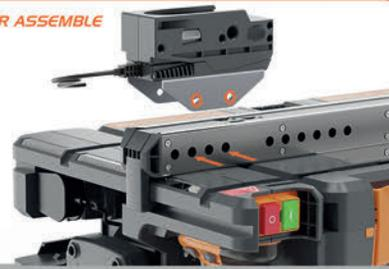
1 Put the Drill-Stand to the Post/Fence locked on the table Surface
