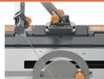
6 measure the cutting angle with the Protractor,
