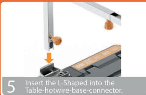
**5** Insert the L-Shaped into the Table-hotwire-base-connector.
