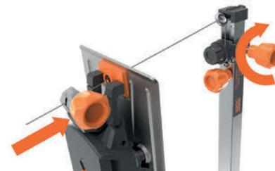
**8** press the spring-loaded wire holder (2 aluminum blocks), while turning the wheel to wind a little length of wire back to wheel to increase the tension of the wire.
