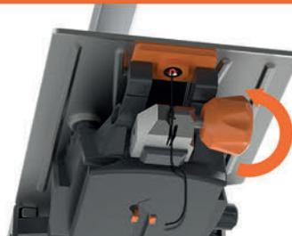
**7** Passing the wire between the gap of the 2 aluminum blocks, then tighten the screw by turning the knob.
