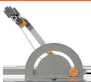
5 measure the cutting angle with the Protractor,
