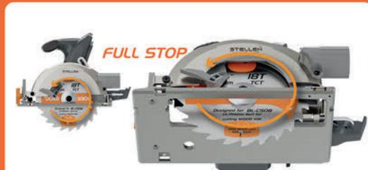
3 rotate the spring-loaded Table Saw Shield fully to the stop position.
