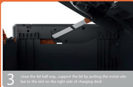
**3** close the lid half way, support the lid by putting the metal side bar to the slot on the right side of charging dock
