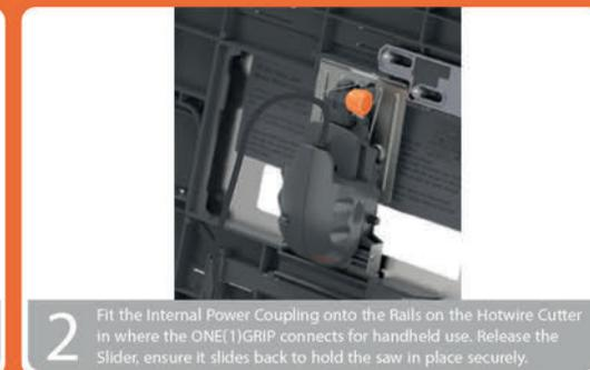
**2** Fit the Internal Power Coupling onto the Rails on the Hotwire Cutter in where the ONE(1)GRIP connects for handheld use. Release the Slider, ensure it slides back to hold the saw in place securely.
