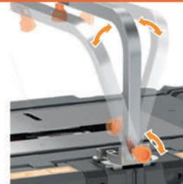
4 measure the cutting angle with the Protractor,
