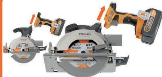
1 remove any ONE(1)Grip and battery from the Circular Saw
