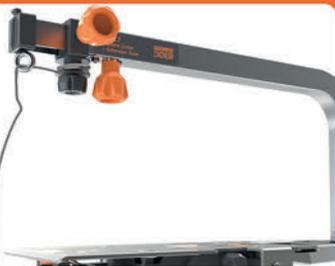
**5** Unwind the cutting wire by turning the wheel until enough wire to pass through the hole.
